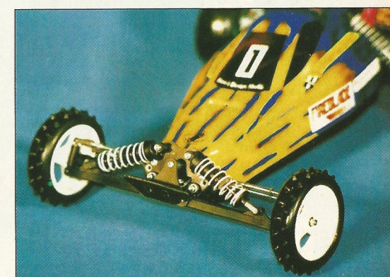
The laydown front shock absorbers allow a very low bodyline.
