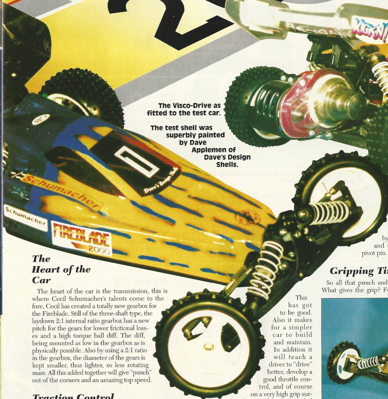
The laydown front shock absorbers allow a very low bodyline.
