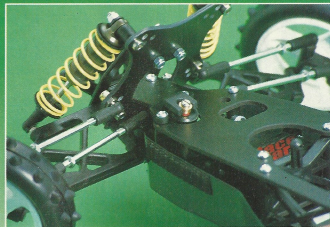
The extended servo saver shaft is now braced at the top by a plastic moulding. Rough tracks - no problem! Short shocks are now used at the front.
