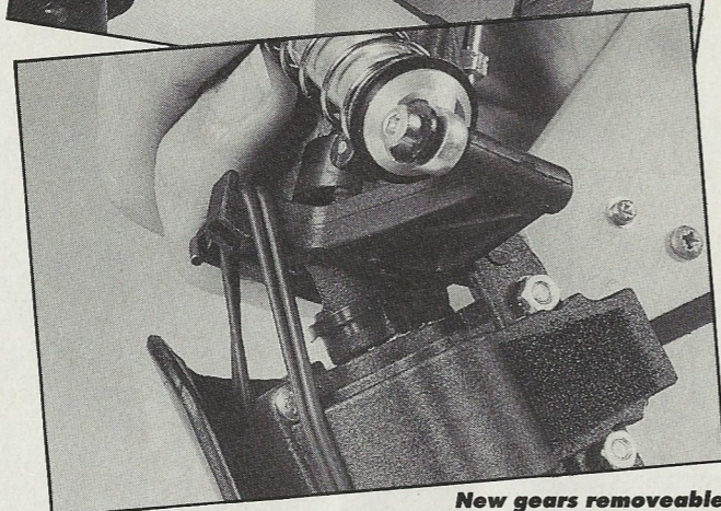
New gears removable without disturbing slipper clutch. Crashback in action is a real suspension saver.
