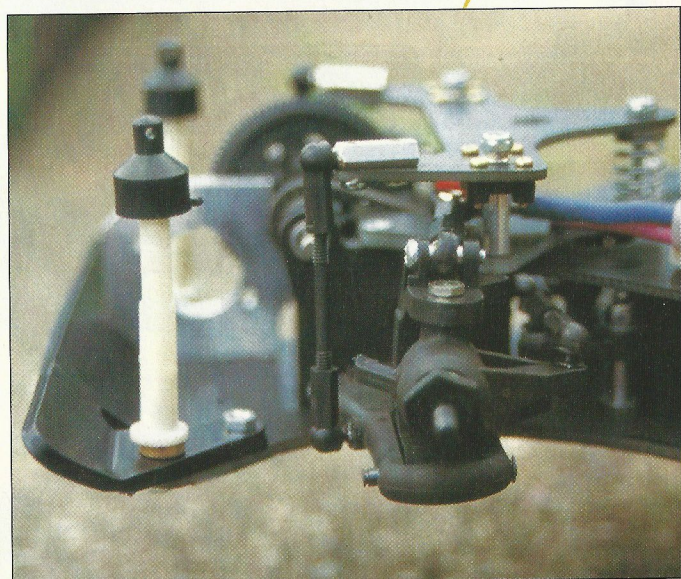
Front suspension detail. The push-rod from the lower wishbone can be clearly seen.
