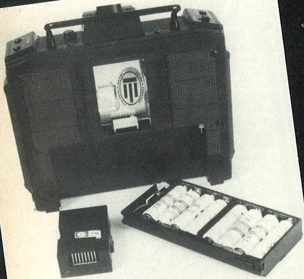
The eight Ni-cads and module are easily removed.
