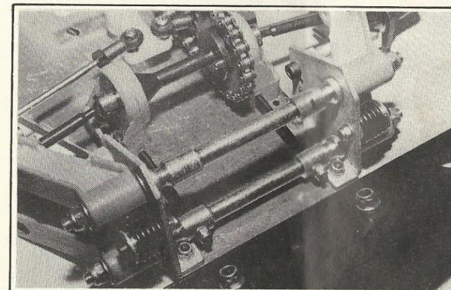
Left: suspension springing on the front-end is via 'hairpin' springs attached to the lower wishbones. Chain adjustment is simple, two threaded adjuster rods pull the bearing blocks forwards on slotted mounts.
