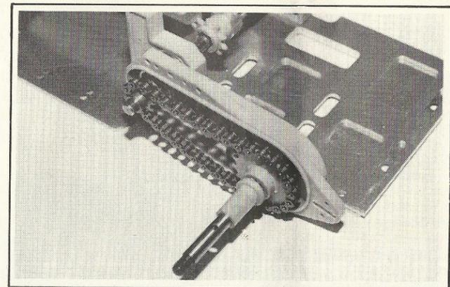
Left: the rear suspension system needs no drive shafts by using the method shown here. When attaching both halves of the trailing arm, seal the joint with silicone rubber compound.
