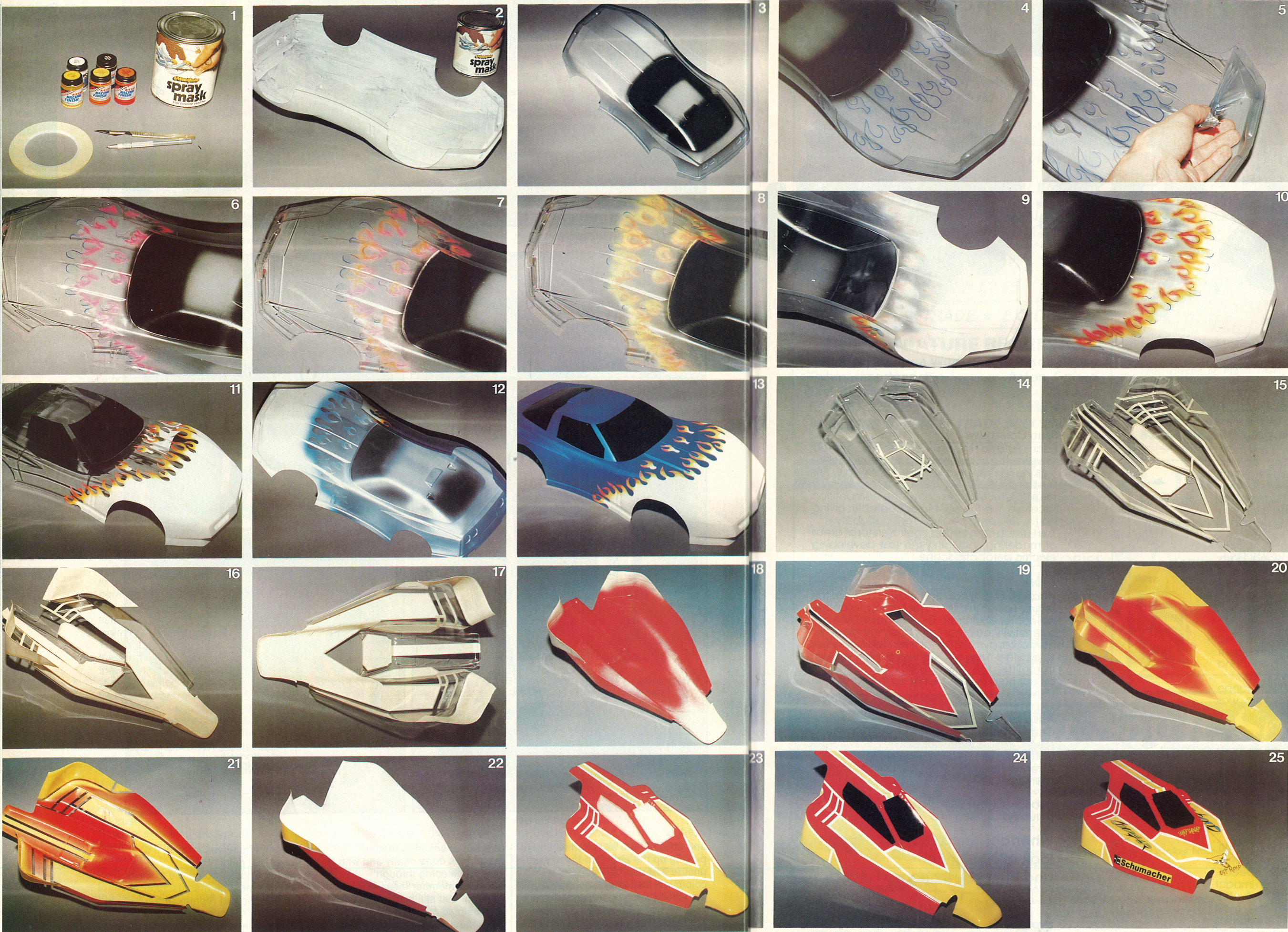
Photo 1: Typical tools and materials required to paint Lexan car bodies. Graphic swivel knife shown in the foreground. 2: Trimmed and washed body is coated with brush-on masking fluid. 3: Dry masking fluid removed and the windows sprayed with metallic black. 4: Custom flame outline drawn on the inside of the shell using a felt-tipped pen. 5: Flame outline cut and masking fluid removed from the bonnet. 6: Fluorescent red paint sprayed into the tips of each flame, working from front to back allowing the overspray to fall on the masked areas of the body. 7: Moving further back into each flame with fluorescent orange. 8: Thinned yellow sprayed to the base of each flame, backing the orange and red. 9: After a careful check that no specks of colour have appeared on the bonnet, the front of the Corvette is sprayed white, 10: From the outside, the results can be seen before removing the masking fluid, and after in photo 11. 12: The remainder of the shell is now sprayed with metallic blue and backed with a light coat of silver. 13: Completed paintwork, prior to adding the decals. 14: Masking the Cougar's window outline with Fine Line tape. 15: Windows backed with paper tape and all colour divides and pinstripes masked with Fine Line. 16 and 17: All areas to be painted yellow masked with paper tape. 18: Red sprayed with light, even coats. 19: Paper tape carefully removed from all yellow areas. 20: Exposed body painted with yellow. 21: Allow all paint to dry then remove the Fine Line tape divides. 22: Spray the entire body white, backing the red and yellow. 23: How the body should look at this stage. 24: All remaining tape removed, the windows sprayed black and all decals added. Useful addresses: Airbrushes — Badger, Dept DG, 156 Stanley Green Road, Poole, Dorset, BH15 3BE. Tel: 0202 673757. DeVillbiss, Ringwood Road, Bournemouth, BH11 9LH. Harden Associates (Powermax), Millet Street, Bury, Lancs. Paint — Pactra: All Ripmax stockists. In case of difficulty, contact Ripmax, 241 Green Street, Enfield, EN3 7SJ. Custom Colour; All Parma stockists.
