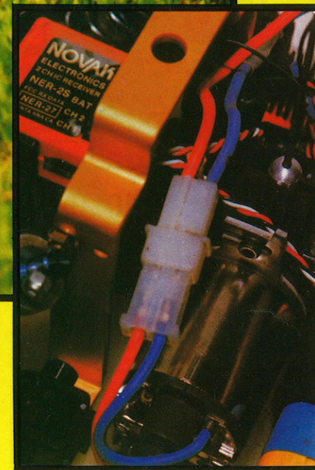
Strong gold anodised roll bar provides protection if the car overturns — note simple motor adjustment.
