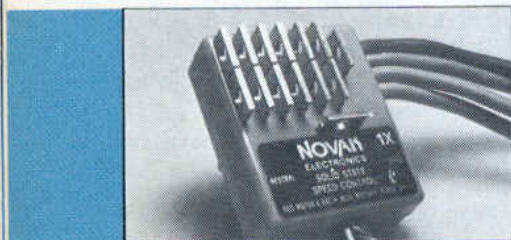
Although the Novak NESC-IX is larger than most competitive speed controls, it provides excellent low-end punch and top speed.
