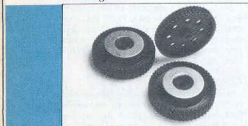
A view of the unassembled diff shows the three separate pulleys. Diff rings are epoxied to the outer pulleys and the inner pulley houses diff balls.
