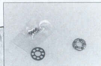
When the original thrust bearing on the left is replaced with the Parma bearing on the right, differential assembly becomes a breeze.
