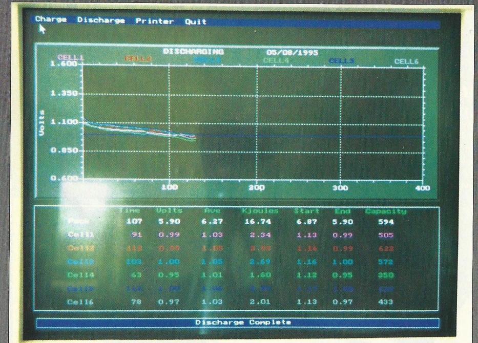
By using the PC link, it is possible to get a thoroughly accurate and graphic picture of the state of each cell in your pack.
