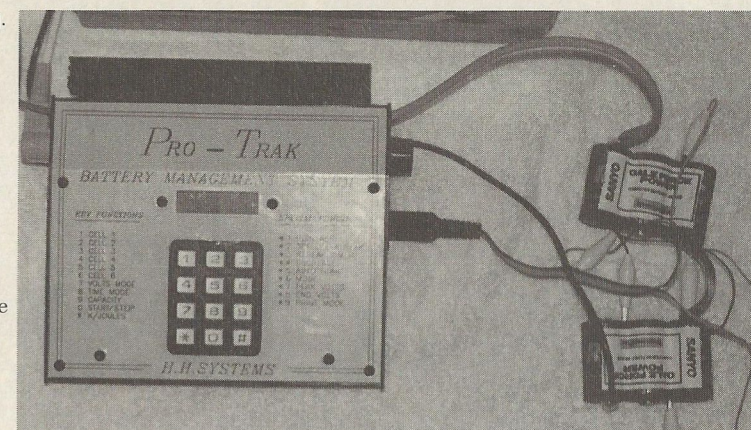
This shot shows the means of individual cell connection.
