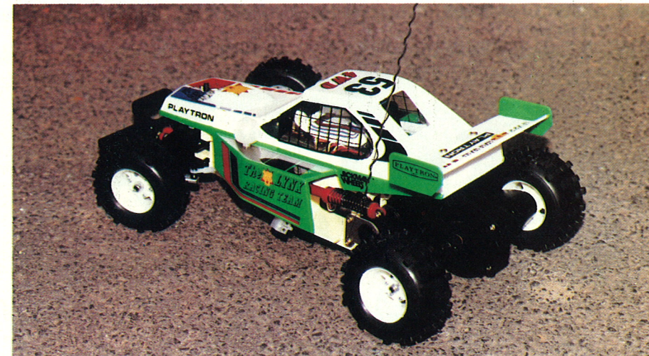
The space frame chassis contributes to a light car. A vented heat sink is fitted to the motor.
