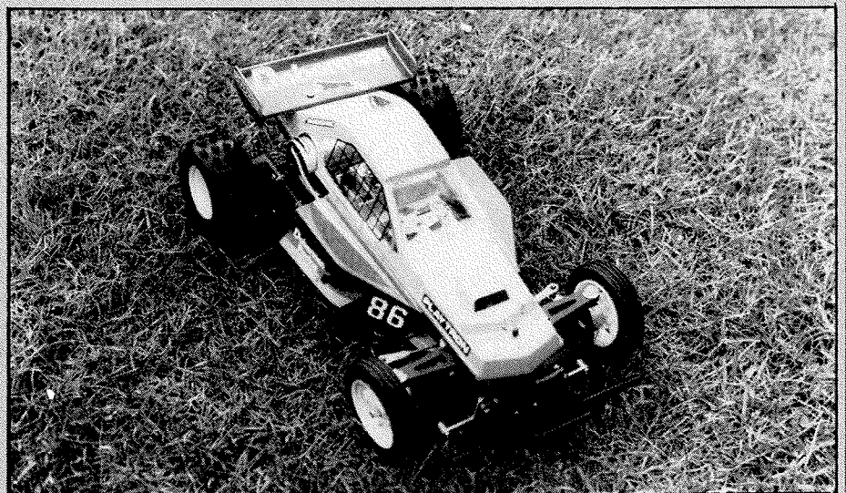
Front suspension uses single monoshock system. Works well but could benefit from an anti-roll bar.
