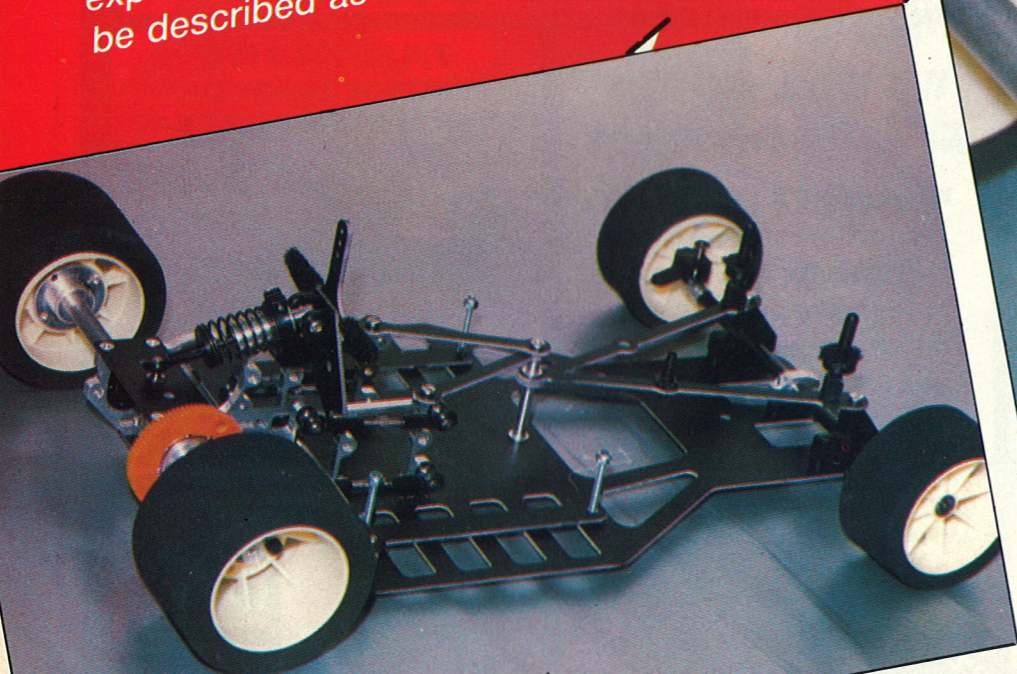
Two triangles give the chassis amazing rigidity yet add nothing to the overall weight.
