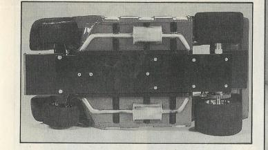
speed controller, the instructions show them only taped on to the underpan we didn't really like this so we have installed them on either side of the car. If you prefer you can make up a GRP plate to sit across the chassis which would provide a much sturdier base for the R/C installation.
