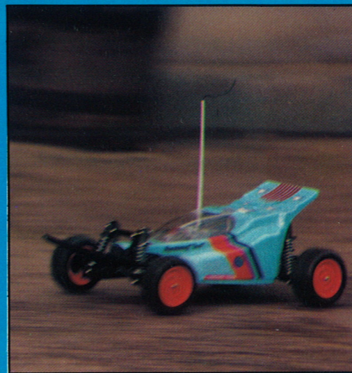
Tall shock towers give a superb amount of movement for the front suspension. New undertray keeps most of the dirt and dust out of the works. At speed, something the ECO does well. All important new rear end giving a range of pre set positions.
