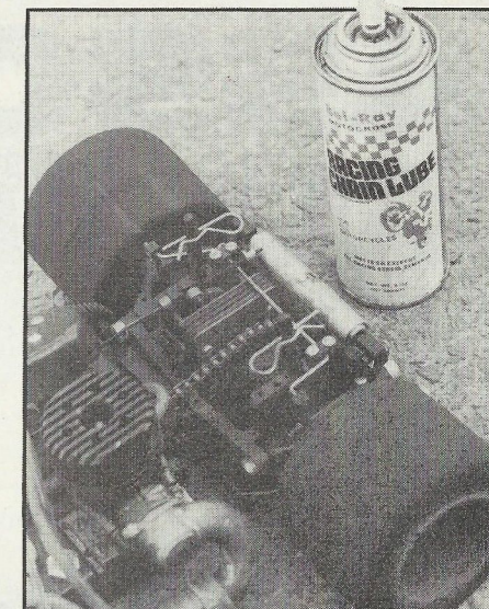
What do you lubricate the drive chain with? Well we found that this motor cycle chain lube was great providing good protection and did not "throw" itself off when racing.
