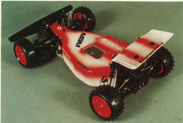
Above: The 'Maxima' comes with a moulded lexan undertray which keeps the mud out by sealing to the bodyshell. Top right: shockers locate to strong towers and onto the arms via self-tapping screws. Right: The car comes complete with a wing and wing mounting kit which works well and does not need to be removed to remove bodyshell.
