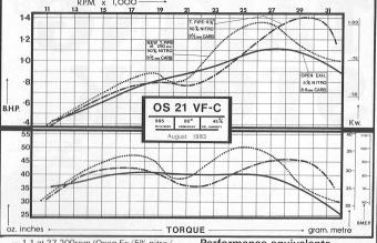
— 1.1 at 27,200rpm (Open Ex/5% nitro/ OS 8.8mm carb).
