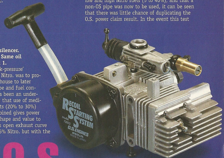
Solid, well engineered crankcase block and base mount combined allowed low vibration levels even at high RPM
