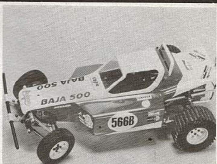
Graupner Kyosho fun 'Wheelin' machine 1/12 electric above left. Above and Below - AYK 1/10 scale buggy could be a serious competitor for the well established Tamiya products. Fully enclosed motor and gear box, shockers and radio box.
