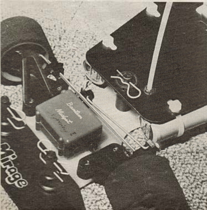
Below left: new Mirage moulded suspension units. Batteries are fitted to a quickly detachable plate for charging, servicing and cooling. This system also makes changes in balance easy to achieve by varying the shape of the battery carrying plate to mount the batteries in differing configurations.
