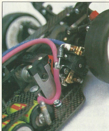
The Cyclone fitted to the author's Yokomo YR4, the power capacitor is mounted in the motor wires. Note the shrink, to protect from "shorts".
