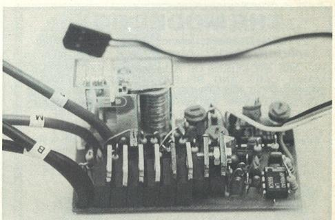
proposition for the manufacturer. Leads are provided for connection to the battery plug and to the motor. A nice touch was the labelling of the leads, confirming the identity of each wire, not leaving the purchaser to sort it all out from a diagram. The controller sent to me arrived with a Futaba connector.
