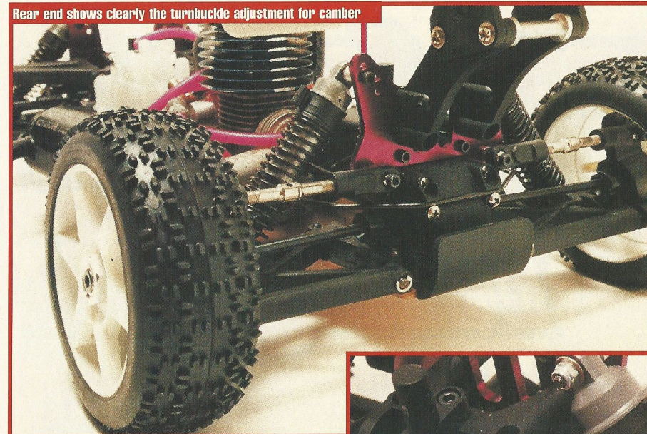
Rear end shows clearly the turnbuckle adjustment for camber
