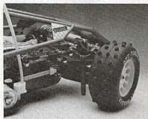
Right front view shows washers on rod ends, servos and antenna mount. Holiday Buggy tires and collars on suspension shafts as well.
