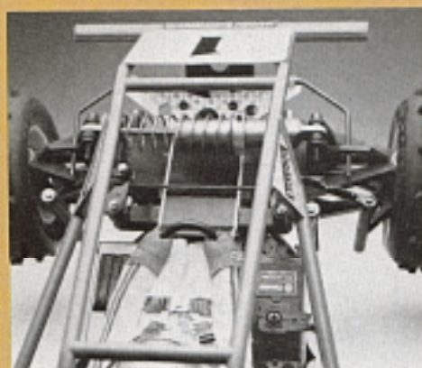
Overhead view showing washers on steering linkage and Delta shock in place.
