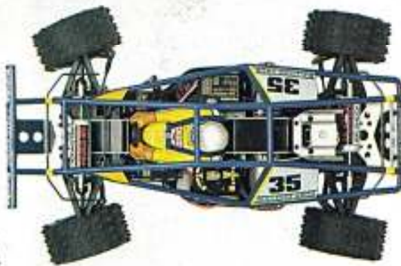
Four wheel steering lets the Bulldog turn sharper and faster than conventional 4x4's.
