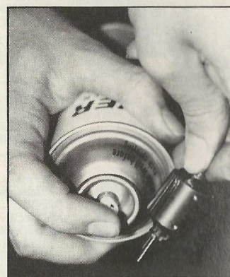
Armature cleaned with motor spray.
