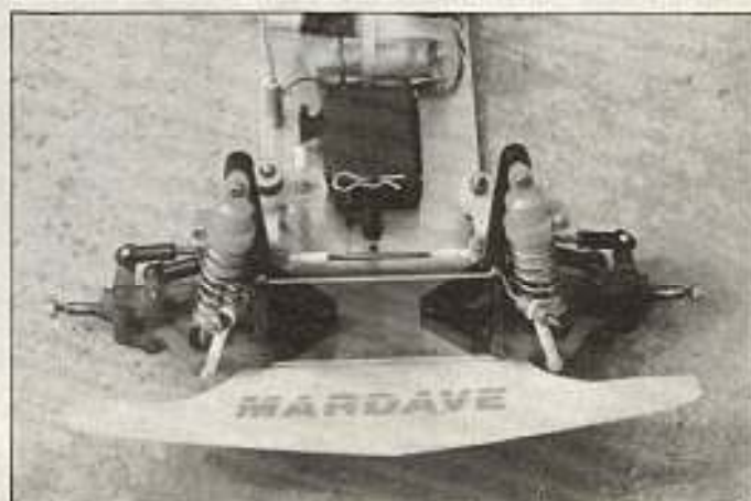
Front shot showing anti-roll bar, RC10 stub axles and parallel link between the servo saver and idler.
