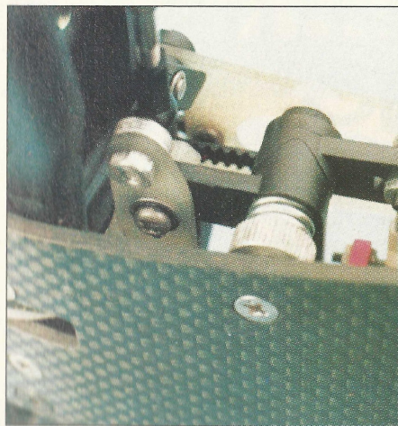
The WCS chassis features a 'kicked up' front to create more ground clearance.
