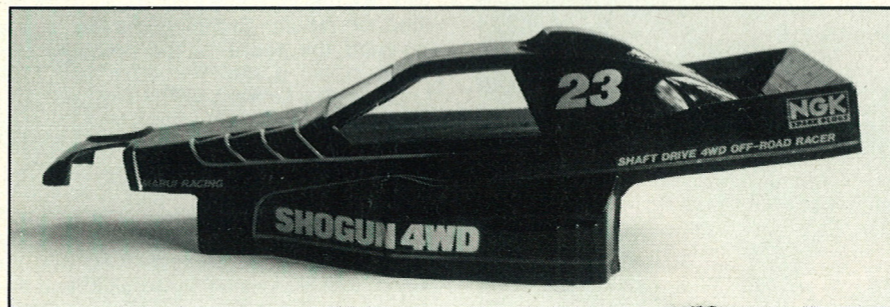
Body shell, note the strengthening moulding around the front shock absorber cut-outs.
