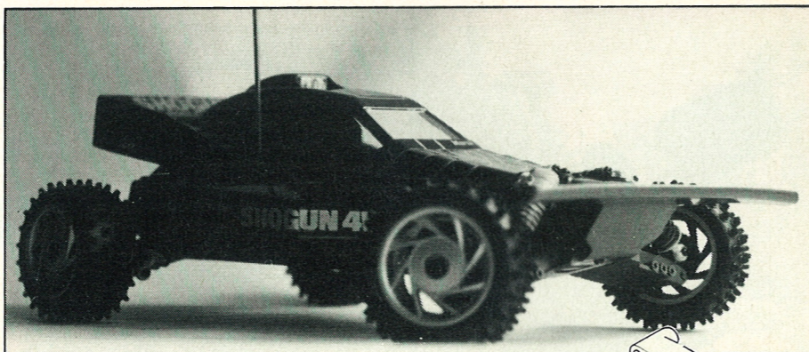
Mean and Lean, note additional front damper positions.
