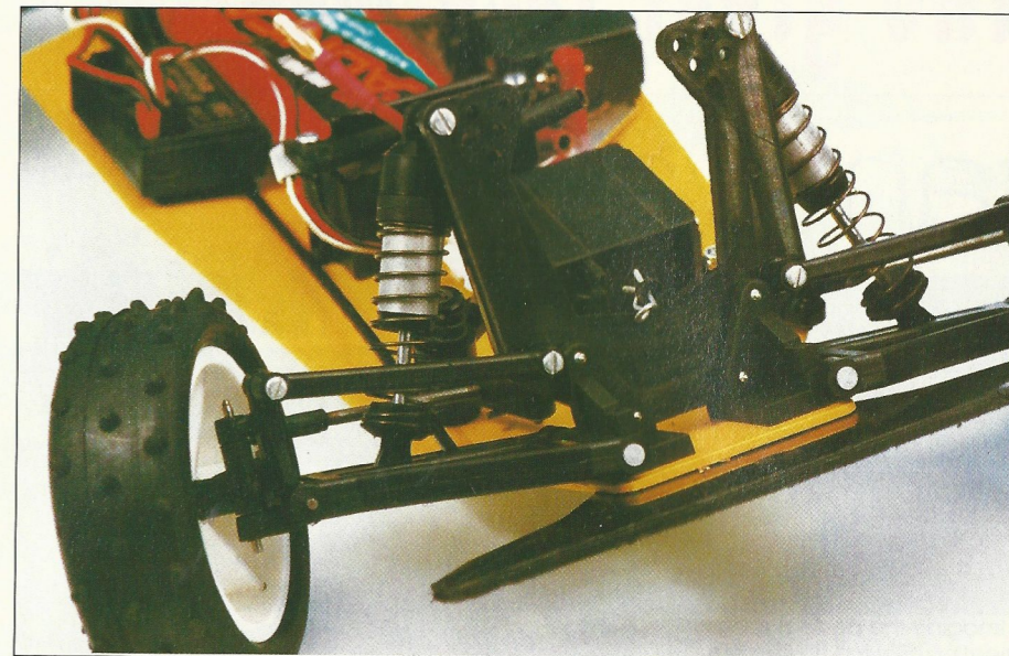
The steering's servo saver benefits from a small nylon or alloy washer placed on the shaft beneath the assembly to reduce friction. This makes the movement smoother.
