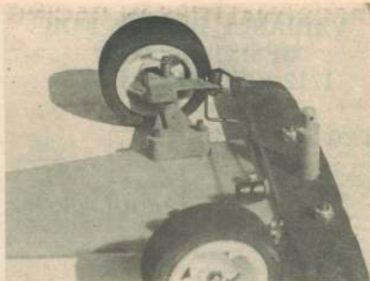
Shims under front of A-frame gives needed caster.
