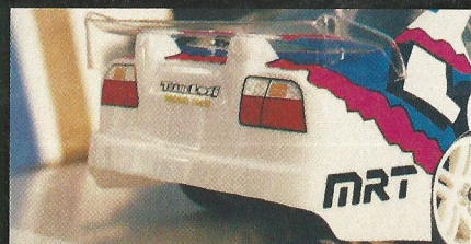
The rear wing didn't quite balance the downforce created by the flat front of the Honda
