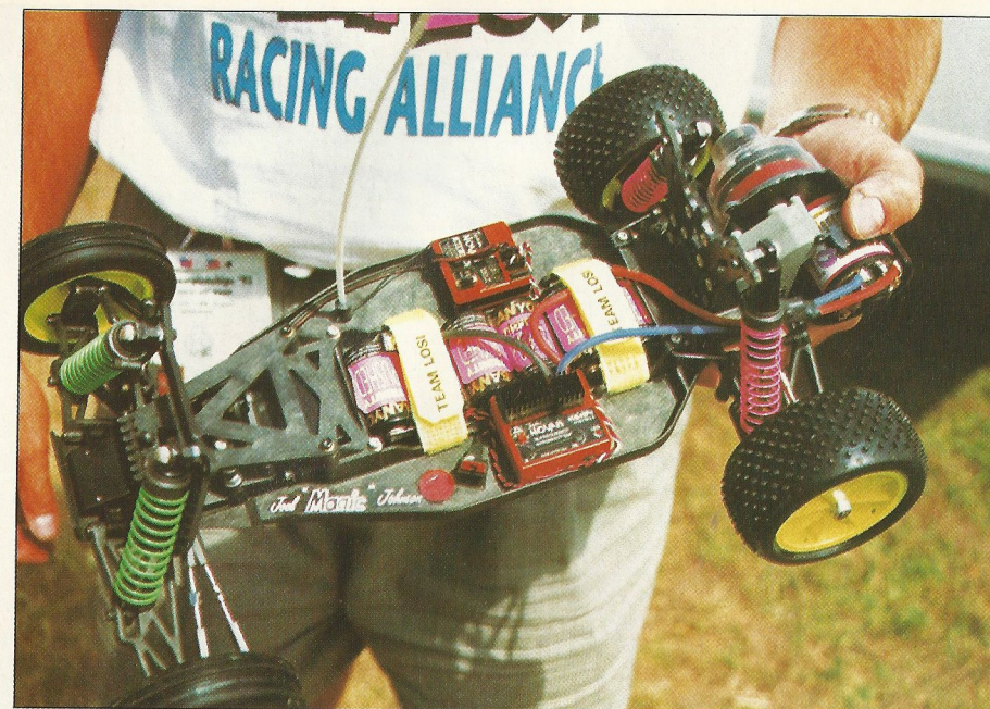
Joel's pre production XX after setting TQ at the World's. Note the rear anti roll bar
