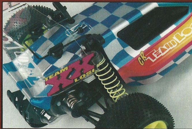
Team Losi's XXCR comes with yellow rear and silver front springs. Also in the kit are the Hydra Drive and the new larger V wing. Below; Could the chassis be any neater? A clean design is very important to the Losi design team. New bodyshell is lower and sleeker than the old XX kit.
