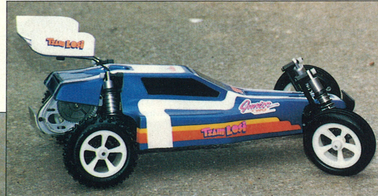
The now famous Losi oil-filled shock absorbers are used on the Junior Two kit.
