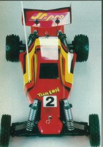
The JRX Pro has the most pink wheels you've ever seen! X pattern tyres on the rear and staggered ribs on the front are the kit items. Neat rear wing mount is clever and lightweight.
