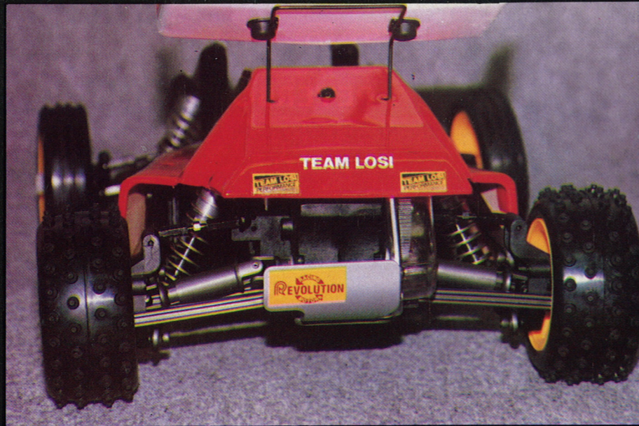
Schumacher type universal drive shafts are employed and are without doubt the best choice.
