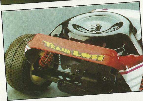
Inside the body shell the car has a neat alloy chassis and OS engine fitted here. Losi made fuel tank sits in the centre for the best possible weight distribution. Red springs are given all round but any of the Losi springs will fit. Car is also capable of using the unique Hydra Drive system.
