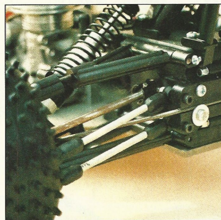
The rear hubs are aligned by two tie bars each side, allowing precise adjustment to the geometry.
