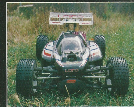
This is the later Diabolo bodyshell, the "bump" covers the front shocks.
