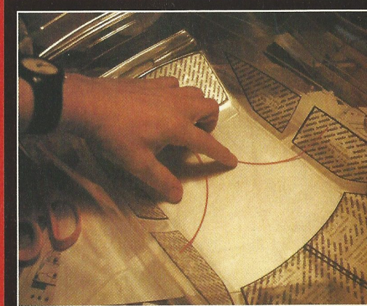
Apply the window masks and start masking off
