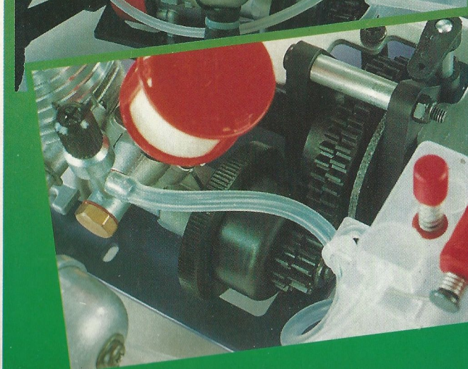
Left; Detail of the two speed centrifugal gearbox unit. Right; Foam air filter and fuel lines all supplied.
