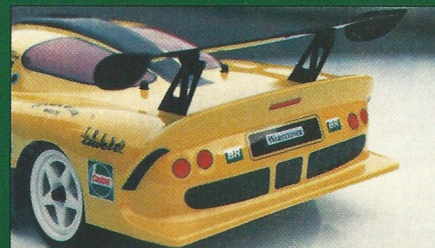
The rear wing is adjustable and with the 'duck tail' gave a lot of downforce.
