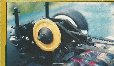
High level layshaft allows a low motor mounting.
