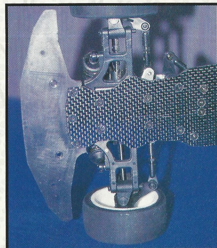
A carbon reinforced chassis come with the kit.
