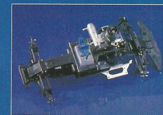
A 75cc fuel tank should give running times of around ten minutes.
