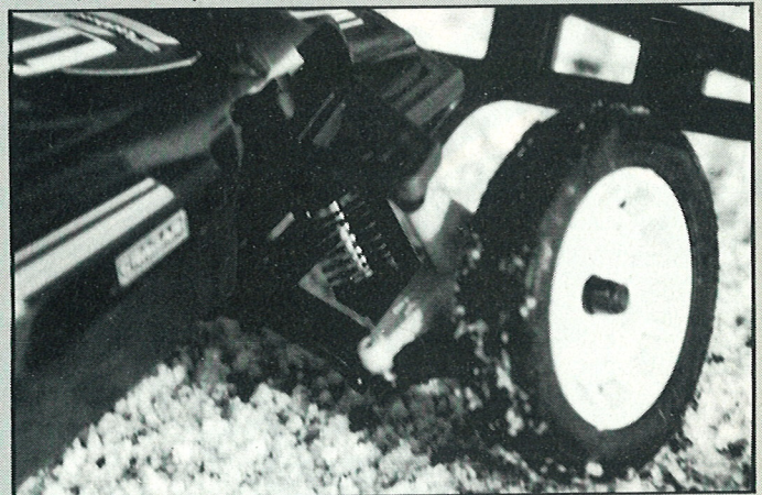
Below, front suspension with its double wishbone system.
