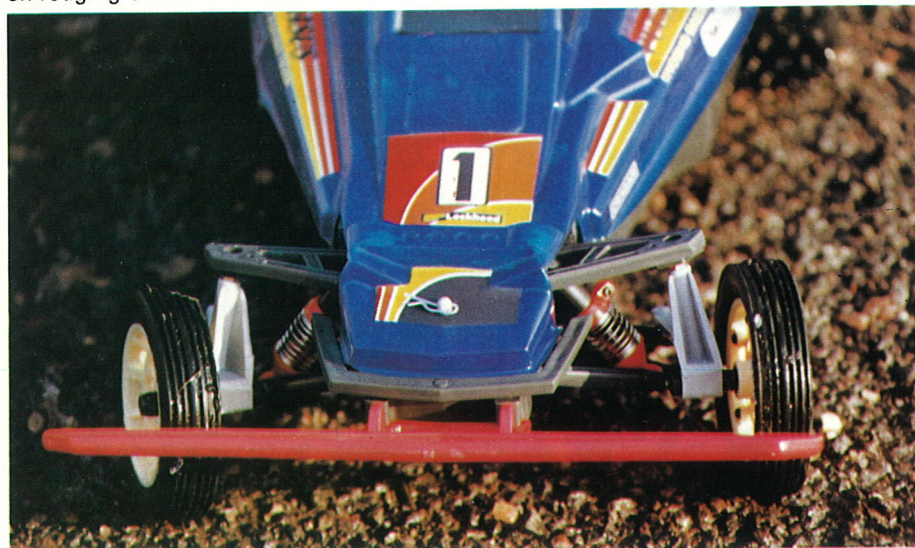
General front suspension detail and ribbed front tyres.
