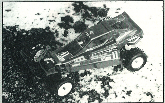
Below, front suspension with its double wishbone system.
