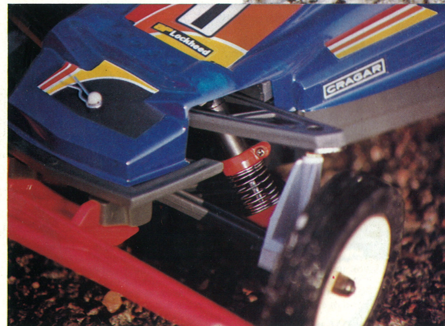
Front suspension is a three part moulding, top and bottom wishbones and a spacer piece. Still very effective.
