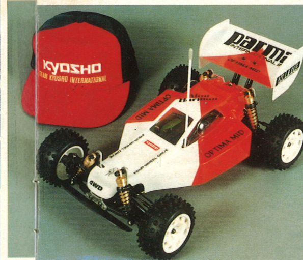
Above: Alain Prost, eat your heart out! Kyosho's latest bodyshell really does the 'mid' proud. Right: Option House shocks are standard as are the 'dot' type tyres. Note - our car has been fitted with battery clamps although the Kyosho tie wrap method works fine.
