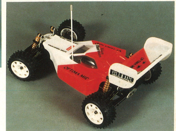
Above: Alain Prost, eat your heart out! Kyosho's latest bodyshell really does the 'mid' proud. Right: Option House shocks are standard as are the 'dot' type tyres. Note - our car has been fitted with battery clamps although the Kyosho tie wrap method works fine.
