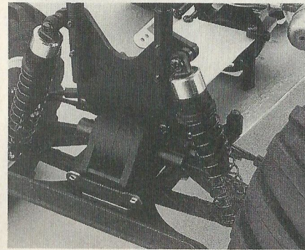
Kyosho have used their excellent plastic dampers that are oil filled and use diaphragms. Below; Kyosho engine complete with pull start system.
