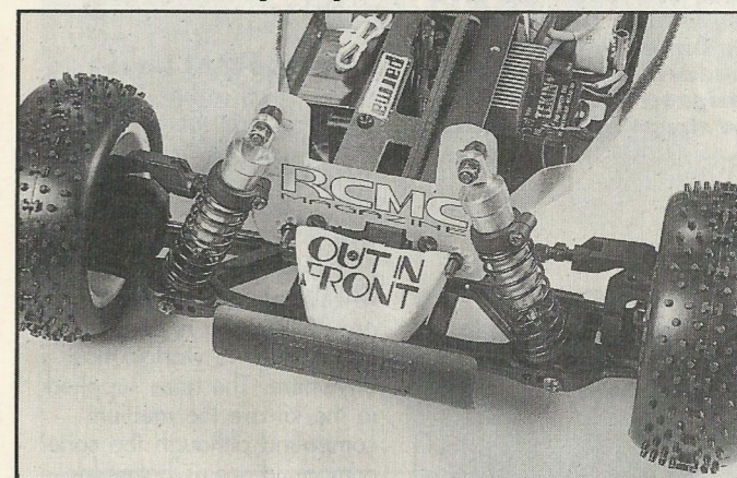
Please note that the car we have used is not totally standard, front shock bracket and chassis have been changed. Our car has also been fitted with Schumacher battery straps.
